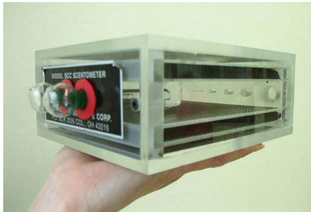
Figure 1. The Scentometer Field Olfactometer (Barnebey Sutcliffe Corp.). Note the two glass nostril ports to the left and the series of orifice holes at the back of the unit to the right in this photo.
