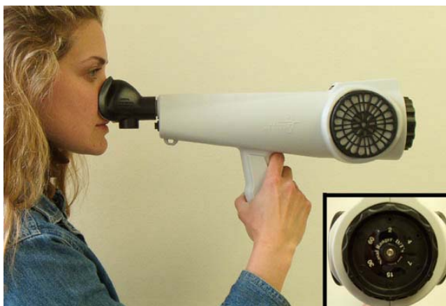
Figure 3. The Nasal Ranger® Field Olfactometer (St. Croix Sensory, Inc.). The inset picture shows a close-up of the orifice dial, which is located to the right side of the Nasal Ranger in this photo.
