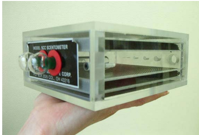
Figure 1. The Scentometer Field Olfactometer (Barneby Sutcliffe Corp.). Note the two glass nostril ports to the left and the series of orifice holes at the back of the unit to the right in this photo.
