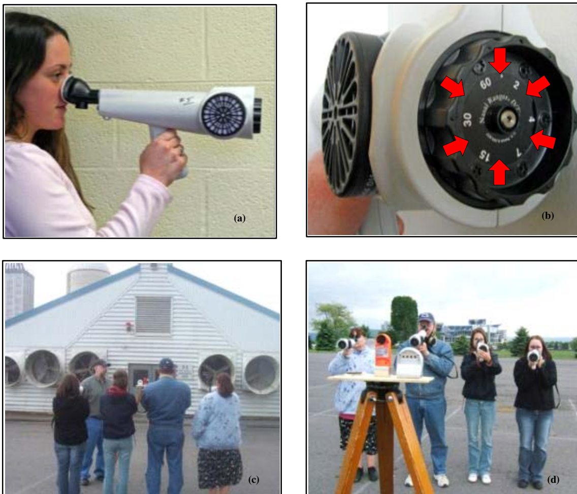
Figure 1. (a) The Nasal Ranger® field olfactometer (NRO) in use. (b) D/T dilution dial located at the air intake end of the unit, which is unseen by the odor assessor during use (100% carbon-filtered air blank positions are located with arrows, between D/T labels). (c) Multiple assessor odor panel facing upwind toward odor source. (d) Multiple assessor odor panel, facing downwind from odor source. Tripod weather station set-up is in foreground.
