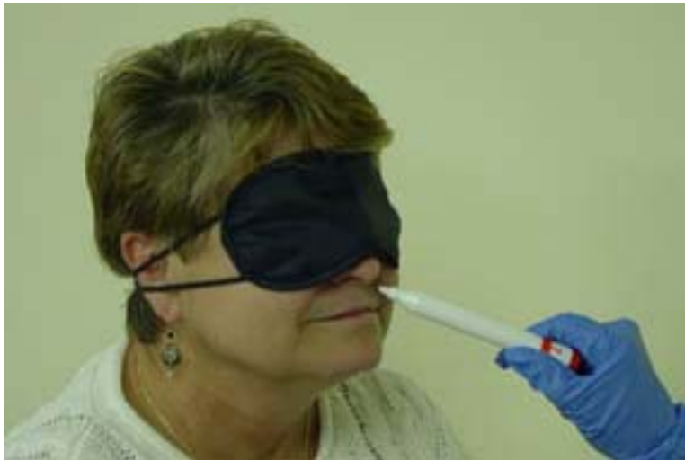
Figure 2. A Test Individual being administered a n-butanol pen from the Odor Pen Kit.
